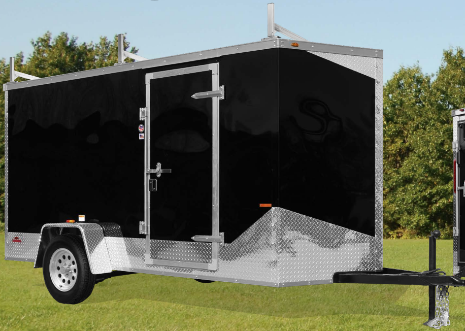
Shown With Optional "Flash Package", Mod Wheels, Screwless Metal and Ladder Racks The "Flash Package" contains the 12" tall ATP on the sides and a flush RV door lock
